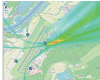
Localization of emissions using TDOA technology
